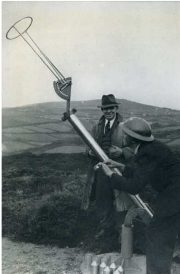
A Holman projector prototype, with anti aircraft sight.
